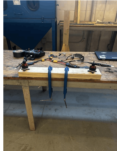
Figure 40: Test apparatus created using scrap wood and clamps. Wires taped to the table to avoid them being caught in the blades.
