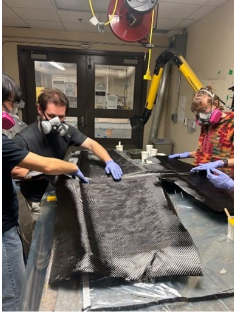
Figure 34: Laying epoxy on the carbon fiber during the layup process.
