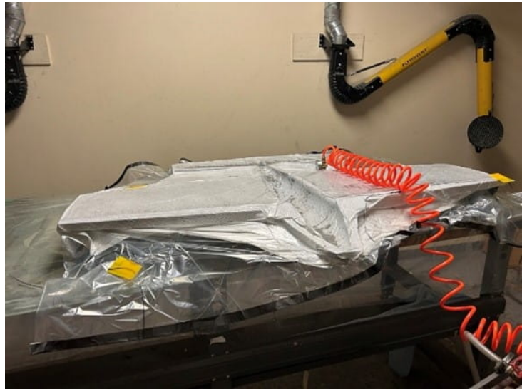
Figure 35: Vacuum seal to allow the degas the epoxy.
